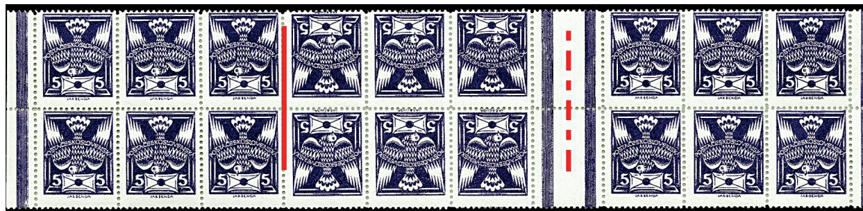
Figure 8. Each set of two rows in a ten-row pane produced three sheetlets. A full pane produced fifteen sheetlets (3 sheetlets x 5 double rows = 15).
