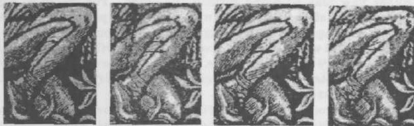
Fig. 10a-d: Progressive Damage to the Shading Lines
