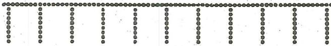
Figure 2: Comb perforations applied to three sides of a stamp in a single stroke.
